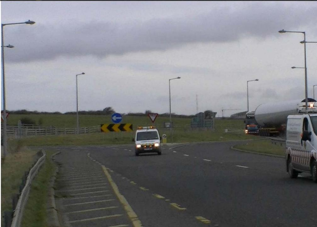
Position taken up to allow swept path cornering at roundabout.
